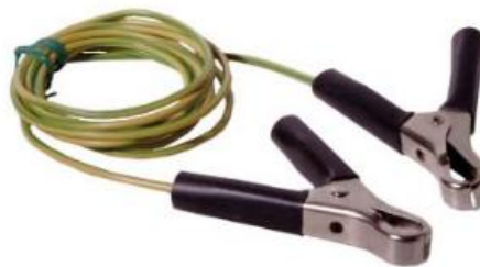
Grounding cable for tank dipping tapes No. 496 Cable dimension 1,5 mm 2 length 2 m with 2 crocodile clamps for grounding of tank dipping tapes to avoid static electricity. Can be used for all tank dipping tapes with brass frames.
